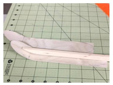
Once the struts are cut out they should match the curve of the ski exactly. Then cut the strut to length.
